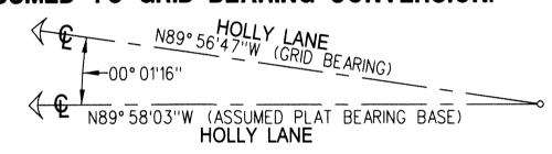
TO CONVERT ASSUMED PLAT BEARINGS TO STATE PLANE GRID BEARINGS ROTATE PLAT BEARINGS 00° 01'16" CLOCKWISE
